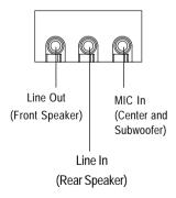
After install onboard audio driver, you may connect speaker to Line Out jack, microphone to MIC In jack. Device like CD-ROM,walkman etc. can be connected to Line-In jack.
