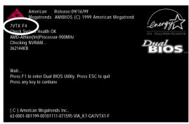
(2) Don't forget to press <DEL> key to enter BIOS setup again when system is boot up. Use the arrows to highlight the item "LOAD SETUP DEFAULTS" then press "Enter". System will ask "Load Setup Defaults (Y/N)?" Press "Y" and "Enter" keys to confirm.
