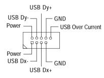
➤ Be careful with the polarity of the front panel USB connector. Check the pin assignment while you connect the front panel USB cable. Please contact your nearest dealer for optional front panel USB 2.0 cable.
