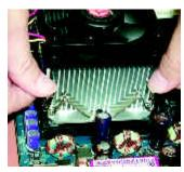
Hook one end of the cooler bracket to the CPU socket first.
