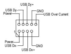
Be careful with the polarity of the front panel USB connector. Check the pin assignment while you connect the front panel USB cable. Please contact your nearest dealer for optional front panel USB cable.
