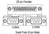
➤ This connector supports 2 standard COM ports and 1 Parallel port. Device like printer can be connected to Parallel port; mouse and modem etc can be connected to Serial ports.
