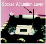
Pull up the CPU socket lever and up to 90-degree angle.
