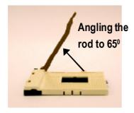
Angling the rod to 65-degree maybe feel a kind of tight, and then continue pull the rod to 90-degree when a noise "cough" made.
