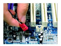
Connect co-axial or optical output to the SPDIF decoder.
