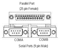
➤ This connector supports 2 standard COM ports and 1 Parallel port. Device like printer can be connected to Parallel port; mouse and modem etc can be connected to Serial ports.
