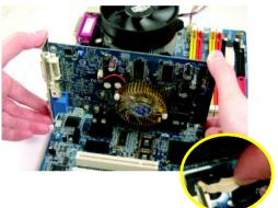
Please align the VGA card to the onboard PCI Express x 16 slot and press firmly down on the slot. Make sure your VGA card is locked by the latch at the end of the PCI Express x 16 slot. When you try uninstall the VGA card, please press the latch as the picture to the left shows to release the card.
