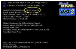
6. Press Del to enter BIOS menu after system reboots. When you are in BIOS menu, move to Load Fail-Safe Defaults item and press Enter to load BIOS Fail-Safe Defaults. Normally the system redetects all devices after BIOS has been upgraded. Therefore, we highly recommend reloading the BIOS defaults after BIOS has been upgraded.
