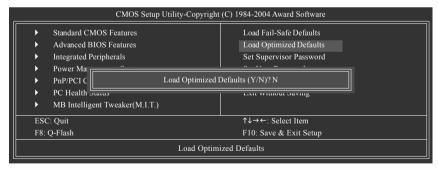
Selecting this field loads the factory defaults for BIOS and Chipset Features which the system automatically detects.
