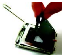
Fig. 2 Remove the plastic covering on the CPU socket.
