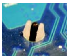
Fig. 5 Please check the back of motherboard after installing. If the push pin is inserted as the picture, the installation is complete.
