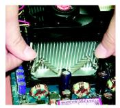
Fasten the cooling fan supporting-base onto the CPU socket on the mainboard.
