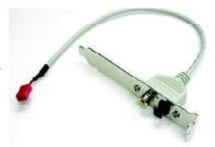
Connect the SPDIF output device to the rear bracket of PC, and fix it with screw.
