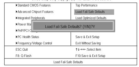
Figure 10: Load Fail-Safe Defaults
