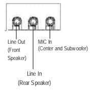
➤ After install onboard audio driver, you may connect speaker to Line Out jack, micro phone to MIC In jack.
