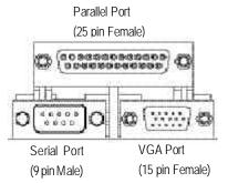
This mainboard sutports 1 standard COM port, 1 VGA port and 1 LPT port. Device like printer can be connected to LPT port; mouse and modem etc can be connected to COM port.
