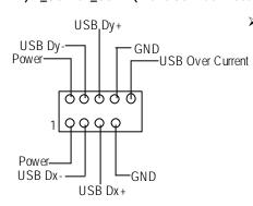
Be careful with the polarity of the front USB connector. Check the pin assignment while you connect the front USB cable.
