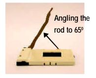
Angling the rod to 65-degree may be feel a kind of tight, and then continue pull the rod to 90-degree when a noise "cough" made.
