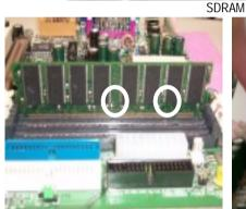
1. The DIMM slot has two notch, so the DIMM memory module can only fit in one direction.
