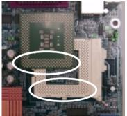
2. The notched corner should point toward the end of the lever. The CPU will only fit in the orientation as shown.
