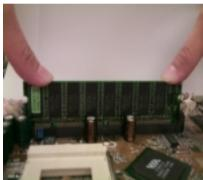
2. Insert the DIMM memory module vertically into the DIMM slot. Then push it down.
