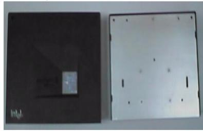
Figure 2: Pentium® II/III XEON SLOT2 Processor
