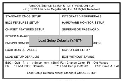
Figure 8: Load Setup Defaults
