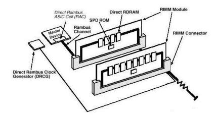
Introduce RIMM (Rambus In-line Memory Module)
