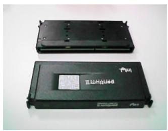
Figure 2:OEM Pentium® II Processor
