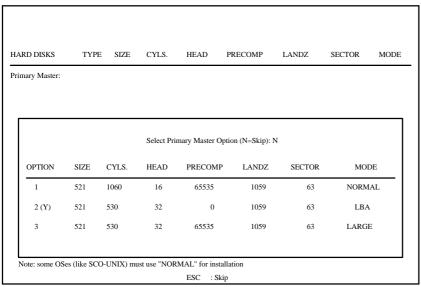
Figure 4.11: IDE HDD Auto Detection
