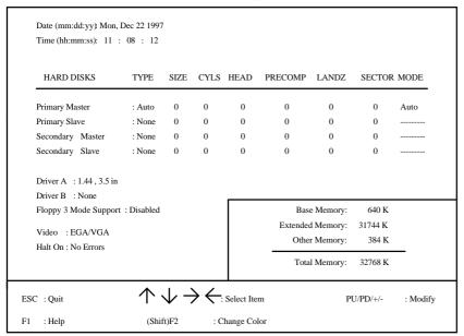
Figure 4.2: Standard CMOS Setup Menu
