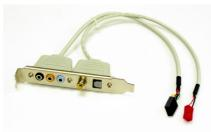
STEP 1 : Secure the Audio Combo Kit at the panel on the back of the case.
