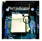
Locate Pin 1 in the socketand look for a (golden) cut edge on the CPU upper corner. Then insert the CPU into the socket
