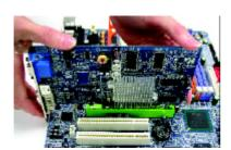
Please align the AGP card to the onboard AGP PRO slot and press firmly down on the slot.
