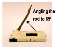
Angling the rod to 65-degree maybe feel a kind of tight, and then confinue pull the rod to 90-degree when a noise "cough" made.
