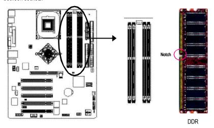
GA-8IG1000 Series supports the Dual Channel Technology. After operating the Dual Channel Technology, the bandwidth of Memory Bus will add double up to 6.4GB/s.
