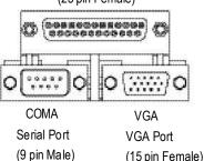
This connector supports 1 standard COM port, 1 Parallel port and 1 VGA port. Device like printer can be connected to Parallel port; mouse and modem etc can be connected to Serial ports.
