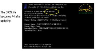
6. Press Del to enter BIOS menu after system reboots and "Load BIOS Fail-Safe Defaults". See how to Load BIOS Fail-Safe Defaults, please kindly refer to Step 6 to 7 in Part One.
