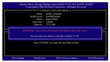
After the completion, you will see the detailed information about the RAID, such as RAID level, disk block size, disk name and disk capacity, etc.
