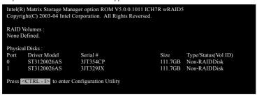
Press Ctrl + I. The Intel RAID Utility - Create RAID Volume window appears (as Figure below).
