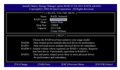
There are four RAID levels: RAID0(Stripe), RAID1(Mirror), RAID 0+1 (Striping + Mirroring) and RAID5. After selecting the RAID level. press **Enter** to select **Strip Size**.
