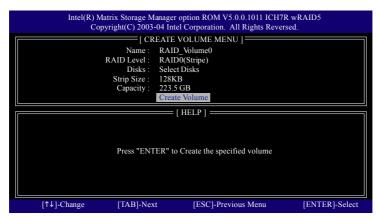
An alert bar will be displayed warning you that all data on selected disks will be lost. Please press Y to complete the set-up of RAID.
