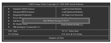
Type "Y" will quit the Setup Utility without saving to RTC CMOS.
