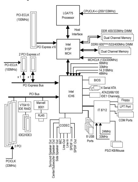
(Note) To use a DDRII 600 memory module on the motherboard, you must install an 800MHz FSB processor and overclock in BIOS.
