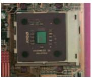
Press down the CPU socket lever and finish CPU installation.
