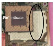
2. Locate Pin 1 in the socket and look for a (golden) cut edge on the CPU upper corner. Then insert the CPU into the socket.
