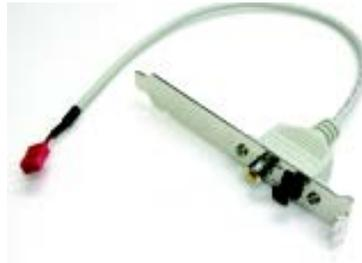
1. Connect the SPDIF output device to the rear bracket of PC, and fix it with screw.
