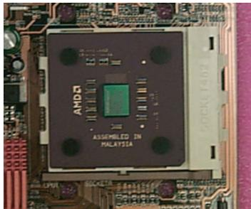
1. Press down the CPU socket lever and finish CPU installation.
