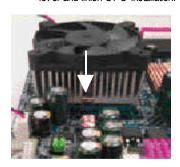
Fasten the heatsink supporting-base onto the CPU socket on the mainboard
