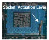
1. Pull up the CPU socket level and up to 90-degree angle.
