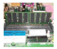
The DIMM slot has two notch, so the DIMM memory module can only fit in one direction.
