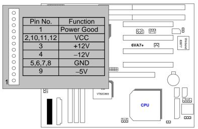
ATX Power : ATX Power Connector
