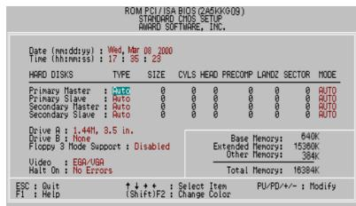
Figure 4.2: Standard CMOS Setup Menu
