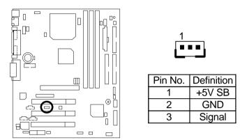
J7: TEL: The connector is for Modem with internal voice connector
