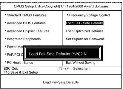
Figure 11: Load Fail-Safe Defaults
