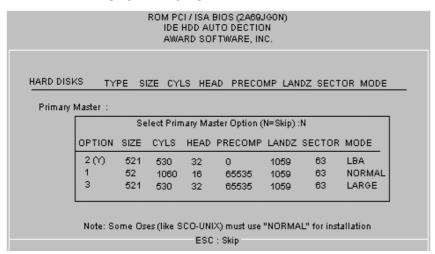
Figure 4.11: IDE HDD Auto Detection
