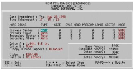
Figure 4.2: Standard CMOS Setup Menu
