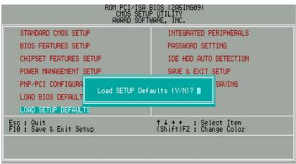
Figure 4.8: Load Setup Defaults
