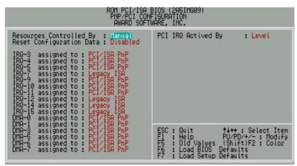
Figure 4.6:PCI Slot Configuration
