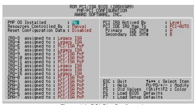
Figure 4.6: PCI Slot Configuration
