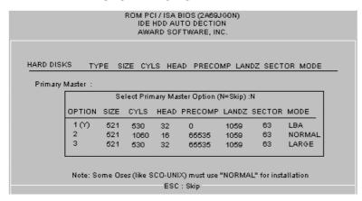
Figure 4.11: IDE HDD Auto Detection
