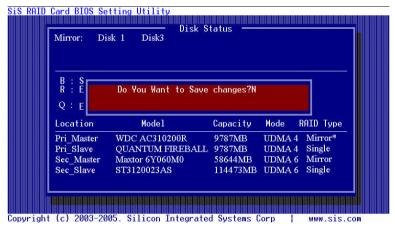
8. Once the array has been created, you will need to FDISK and format the array as if it were a new single hard drive.
