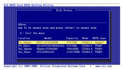
Press <N> and <Enter> to Create Mirror only. (If Press <Y> and <Enter>, it will Duplicate the data on source disk to mirror disk)
