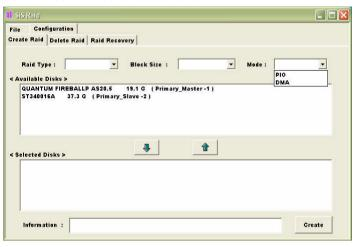
d) Available Disks: This pane will list out all the disks that can be used to create a RAID set currently. It will show some disk information (ex. Location, serial numbers, the ability of boot and the status of recovering).
