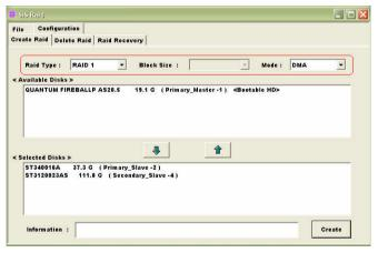
NOTE: The RAID1 array supports two hard disks only.
