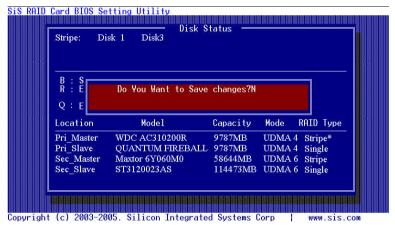
Once the array has been created, you will need to FDISK and format the array as if it were a new single hard drive.
