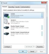
In Windows 7, select Start>Control Panel>Hardware and Sound>Sound>Playback, set Intel(R) Display Audio to the default playback device.
