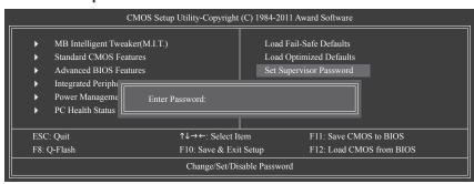
Press <Enter> on this item and type the password with up to 8 characters and then press <Enter>. You will be requested to confirm the password. Type the password again and press <Enter>.
