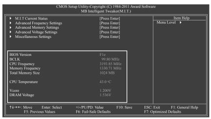
This section provides information on the BIOS version, CPU base clock, CPU frequency, memory frequency, total memory size, CPU temperature, Vcore, and memory voltage.
