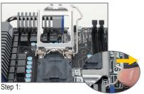
Gently press the CPU socket lever handle down and away from the socket with your finger. Then completely lift the CPU socket lever and the metal load plate will be lifted as well.
