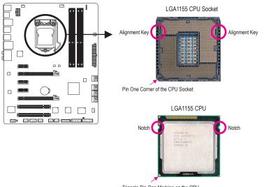
B. Follow the steps below to correctly install the CPU into the motherboard CPU socket.
