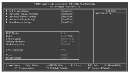
This section provides information on the BIOS version, CPU base clock, CPU frequency, memory frequency, total memory size, CPU temperature, Chipset temperature, Vcore, and memory voltage.
