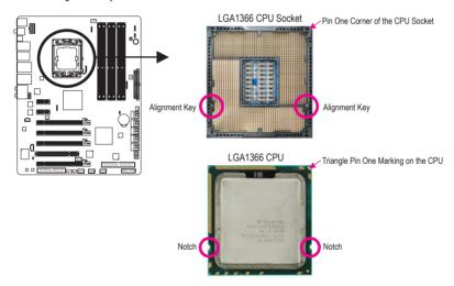
B. Follow the steps below to correctly install the CPU into the motherboard CPU socket.
