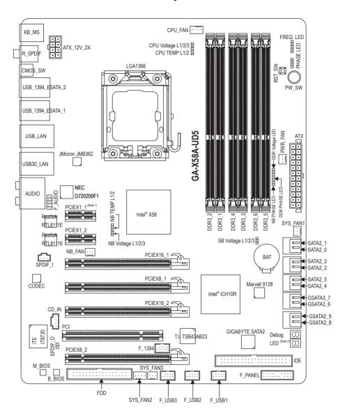
(Note 1) Due to a hardware limitation, the PCIEX1\_1 slot can only accommodate a shorter PCI Express x1 expansion card. For a longer expansion card, use other expansion slots.
