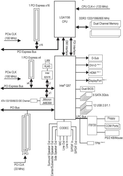
(Note 1) You can use only one of the onboard digital graphics ports (DisplayPort, HDMI, and DVI-D) for output when in the BIOS Setup program or when during the POST screens.
