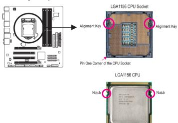
Triangle Pin One Marking on the CPU
