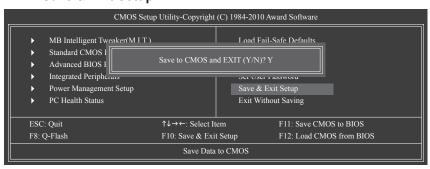
Press <Enter> on this item and press the <Y> key. This saves the changes to the CMOS and exits the BIOS Setup program. Press <N> or <Esc> to return to the BIOS Setup Main Menu.
