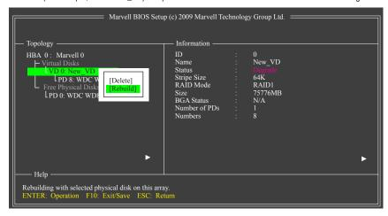
Step 2: The selection bar will move to the new drive. Press the <Space> key to select it and then press <Enter>. When prompted to confirm, press <Y> to begin the rebuild or <N> to cancel.
