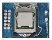
Step 5: Push the CPU socket lever back into its locked position.
