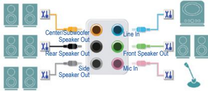
The integrated HD (High Definition) audio provides jack retasking capability that allows the user to change the function for each jack through the audio driver.
