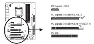
Follow the steps below to correctly install your expansion card in the expansion slot.
