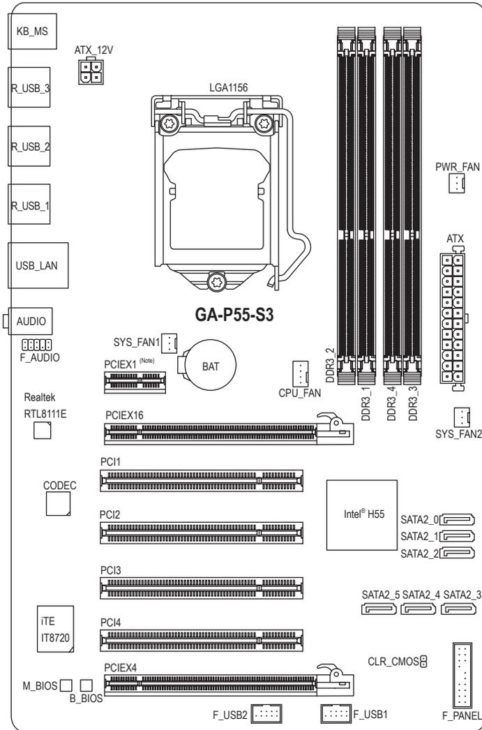
(Note) Due to a hardware limitation, the PCIEX1 slot can only accommodate a shorter PCI Express x1 expansion card. For a longer expansion card, use other expansion slots.
