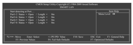
This motherboard incorporates cable diagnostic feature designed to detect the status of the attached LAN cable. This feature will detect cabling issue and report the approximate distance to the fault or short. Refer to the following information for diagnosing your LAN cable:
