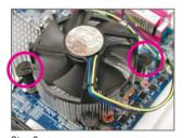
Step 3: Place the cooler atop the CPU, aligning the four push pins through the pin holes on the mother-board. Push down on the push pins diagonally.
