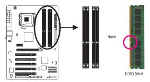
A DDR3 memory module has a notch, so it can only fit in one direction. Follow the steps below to correctly install your memory modules in the memory sockets.
