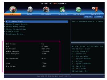
This section provides information on the BIOS version, CPU base clock, CPU frequency, memory frequency, total memory size, CPU temperature, Vcore, and memory voltages.
