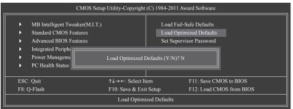
Press <Enter> on this item and then press the <Y> key to load the optimal BIOS default settings. The BIOS defaults settings help the system to operate in optimum state. Always load the Optimized defaults after updating the BIOS or after clearing the CMOS values.
