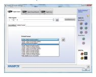
(Note) If you have connected a S/PDIF digital audio cable (provided by expansion cards) to the 2-pin S/PDIF Out header (SPDIF\_O) on the motherboard to output digital audio to your expansion card, you can enter the Digital Output(Optical) screen to configure further settings, such as the sample rate and bit depth.
