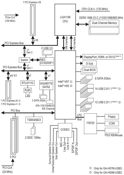
(Note 1) You can use only one of the onboard digital graphics ports (e.g. DisplayPort, HDMI, and DVI-D) for output when in the BIOS Setup program or when during the POST screens.
