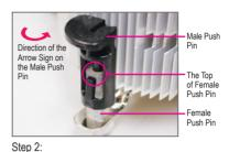
Before installing the cooler, note the direction of the arrow sign on the male push pin. (Turning the push pin along the direction of arrow is to remove the cooler, on the contrary, is to install.)
