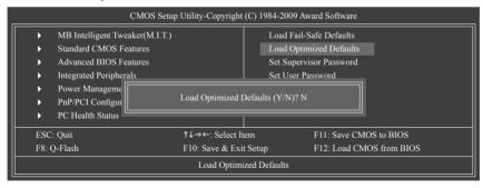
Press <Enter> on this item and then press the <Y> key to load the optimal BIOS default settings.
