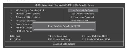
Press <Enter> on this item and then press the <Y> key to load the safest BIOS default settings. In case system instability occurs, you may try to load Fail-Safe defaults, which are the safest and most stable BIOS settings for the motherboard.
