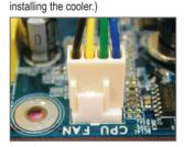
Finally, attach the power connector of the CPU cooler to the CPU fan header (CPU\_FAN) on the motherboard.
