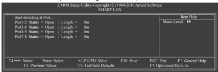
This motherboard incorporates cable diagnostic feature designed to detect the status of the attached LAN cable. This feature will detect cabling issue and report the approximate distance to the fault or short. Refer to the following information for diagnosing your LAN cable:
