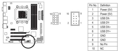
When the system is in S4/S5 mode, only the USB ports routed to the F\_USB1 header can support the ON/OFF Charge function.
