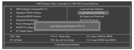
Press <Enter> on this item and then press the <Y> key to load the optimal BIOS default settings.
