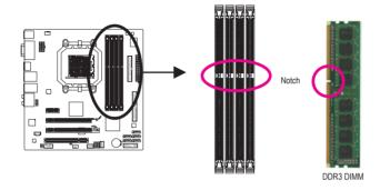
A DDR3 memory module has a notch, so it can only fit in one direction. Follow the steps below to correctly install your memory modules in the memory sockets.
