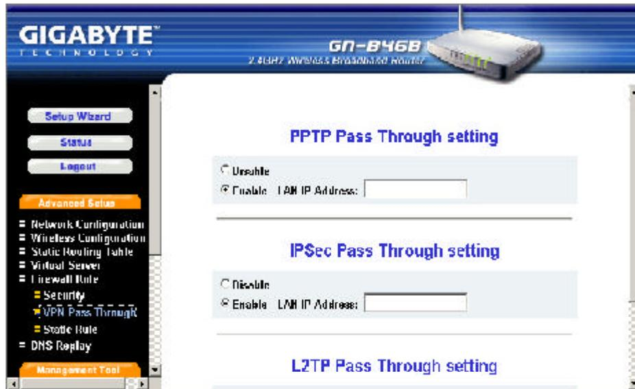
Virtual private networks (VPN) are secured private network connections, built on top of publicly-accessible infrastructure, such as the Internet or the public telephone network. VPNs typically employ some combination of encryption, digital certificates, strong user authentication and access control to provide security to the traffic they carry. They usually provide connectivity to many machines behind a gateway or firewall.
