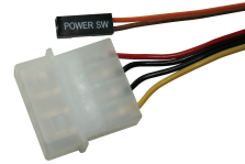
f. Motherboard 2-pin connector and 4-pin connector to power supply.
